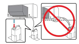
Make sure that the tube sits above the yellow line indicated on the outside of the bottle. If the tube is too long, cut the end to the appropriate length.
