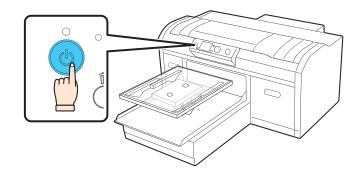
Caution: Do not turn off or unplug the printer while the blight is flashing. Also, do not open the ink covers during the charging process
