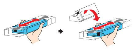
2 Open the ink covers and install each cartridge into the correct slot for its color.
