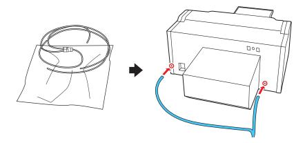
Attach the two tube clamps to the left and right sides on the back of the printer and route the waste ink tube through the clamps as shown.
