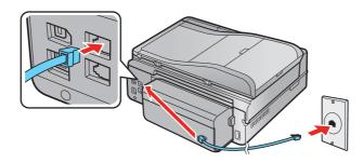
**Note:** If you're connecting to a DSL phone line, you must use a DSL filter or you won't be able to fax. Contact your DSL provider for the necessary filter.
