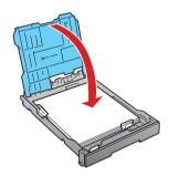
5 Squeeze the edge guides and slide them out. Then insert 4 x 6-inch or 5 x 7-inch photo paper with the glossy or printable side face-down.
