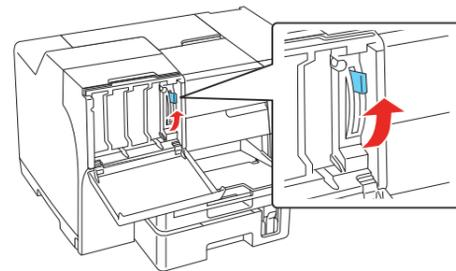
The arrow mark should be on top and pointing toward the printer.
