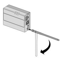
2. Secure the print server to the back of the all-in-one using the included hook-and-loop self stick tape. The antenna should be on left as shown below:
