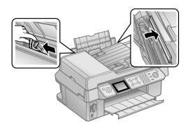
4. Load paper against the right edge guide and behind the tab, with the printable side face up.
