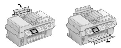
3. Slide the edge guide to the left and flip the feeder guard forward.
