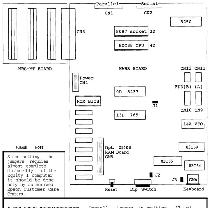
\* NON-EPSON KEYBOARDSUPPORT - Install jumpers in positions J2 and position J3 (Early systems did not have this capability and do not have these jumper positions installed.)
