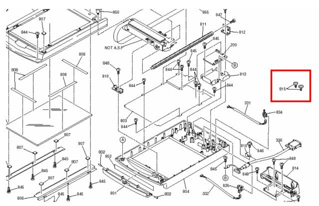
The correct part and reference numbers for the Expression 1600/1680 Transparency Unit (B813182) lock-down thumbscrews are respectively: 1012588 and 815. The Parts Price List (PPL) description is S. THUMB SCREW M4X10 F/NI, Quantity = 2.
