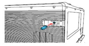
After inserting the Flash drive, press and hold the projectors Power button for 5 seconds while connecting the power cable to the projector.
