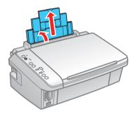
Open the output tray, pull out the extensions, and raise the stopper.
