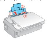
**2** Open the output tray, pull out the extensions, and raise the stopper.
