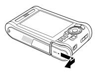
2 Insert the battery into the compartment in the direction of the arrow on the battery.
