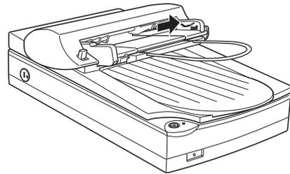
2. Insert the paper stack into the ADF until it meets resistance. Make sure that the side you want to scan is facing up, with the top edge facing into the feeder; the first page you want to scan should be on top. Then move the right edge guide so it is flush with the right edge of your paper.
