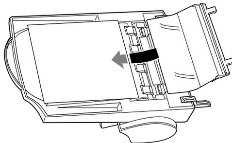
2. Insert the hooks into the rectangular holes in the bottom of the auto document feeder. Make sure the hooks click into place.
