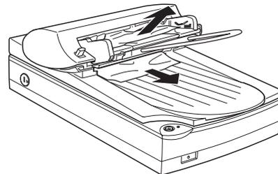
4. If paper is still jammed inside the mechanism, open the cover to remove it.
