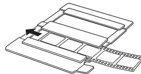
Then place the film holder on the document table. Be sure to align the upper left corner of the film holder with the upper left corner of the transparency unit. You can adjust the position of 35 mm film by sliding the strips in the film holder so the frames you want to scan are positioned in the window.
