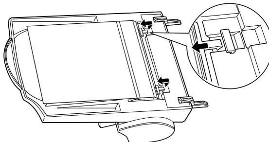
6. Pull the paper path guide upwards and out to remove it.
