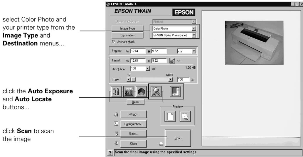
11. When the Advanced EPSON TWAIN window appears, the scanner pre-scans the picture automatically. When it finishes, select these settings:
