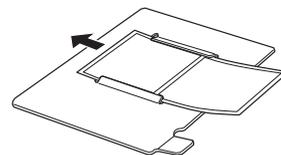
Then place the film holder on the document table. Be sure to align the upper left corner of the film holder with the upper left corner of the transparency unit.
