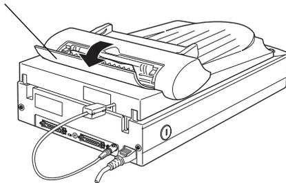
5. After removing jammed paper, make sure that the cover is closed, and push the feeder mechanism down until it clicks into place.
