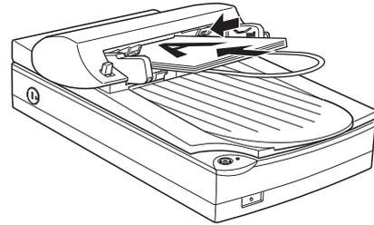
Documents are output into the lower tray after scanning is finished.
