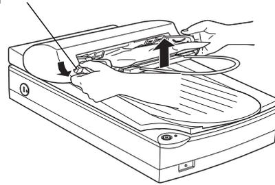
3. Slowly pull the jammed paper out of the feeder mechanism. (Be careful not to pull too hard; the paper may tear, making it more difficult to remove.)
