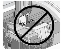
7. Press down firmly on the ink cartridge clamp until it snaps in place.
