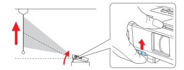
**PowerLite 1775W:** Press the **Focus** buttons to sharpen the image.
