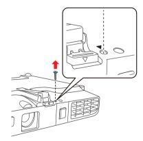
Remove the wireless LAN module cover.
