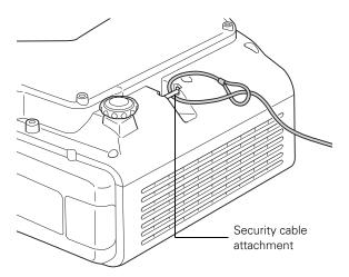
■ Kensington security slot. The security slot (located above the power inlet) is compatible with the MicroSaver security systems manufactured by Kensington. You can purchase this lock from Epson (see page 10).
