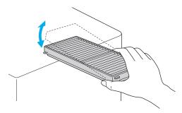
5. To clean any dust remaining on the air filter, use a small vacuum cleaner designed for computers and other office equipment to clean the front. If you don't have one, gently clean the vent with a soft brush (such as an artist's paintbrush).
