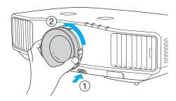
4. Remove the lens by pulling it straight out.
