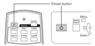
The projector beeps once and the  $\circlearrowleft$  power light flashes green as the projector warms up, then an image begins to appear. When the  $\circlearrowleft$  power light stops flashing and remains green, the projector is ready for use.
