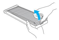
4. With the front of the air filter facing down, tap it four or five times to shake off the dust. Turn it over and tap the other side in the same way to shake off the dust.
