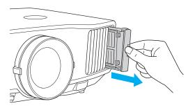
3. Place your finger into the groove and remove the air filter as shown.
