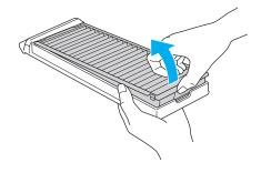
3. Insert the new air filter into the holes in the cover, then press it firmly into place.
