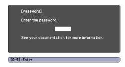
Hold down the Num button on the remote control and use the numeric keypad to enter the four digit password. The password screen closes and projection begins.
