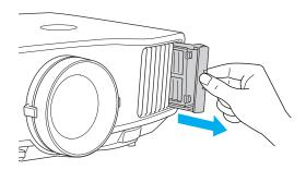
2. Place your finger into the groove and remove the air filter as shown.
