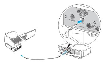
If you have equipment connected to the Video1, Video2, or S-Video ports, connect an RCA audio cable to the L and R Audio (Video) ports.
