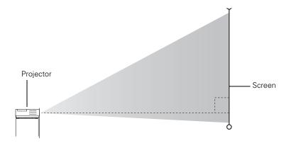
If you place the projector below screen level, you can use the vertical lens shift dial to raise the lens (see page 32). You can also tilt the projector up by extending the front adjustable foot. Tilting the projector causes the image to become "keystone" shaped, but you can correct the distortion (see page 33).
