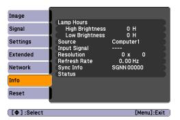
The life span of the lamp is about 2000 hours if the Brightness Control setting in the Settings menu is set to High (default), and 3000 hours if the Brightness Control setting is set to Low. Make sure you have a spare lamp handy if the usage hours on this menu are close to the life span of your lamp.
