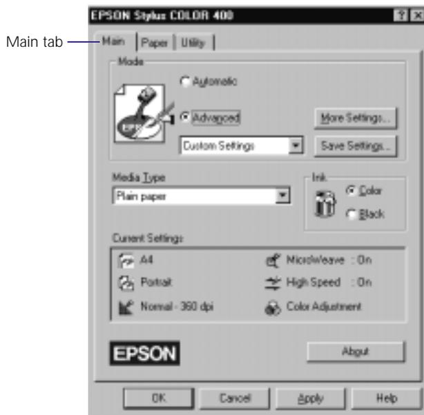
Most of the basic driver settings you'll need to check are on the Main menu. Settings controlling the paper size, orientation, and layout are on the Paper menu. You can run the printer utilities from the Utility menu (see Chapter 4 for details).
