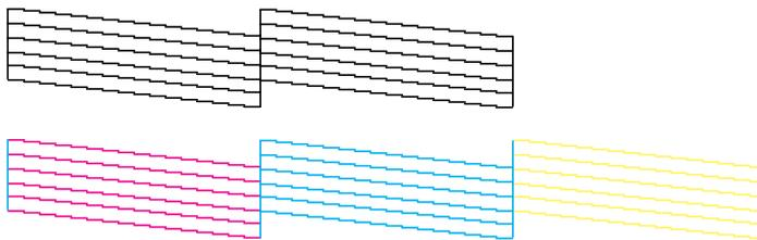
5. To end the check, turn off the printer after it prints the check page. Then reconnect the interface cable and turn on your printer and computer.
