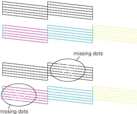
Each staggered horizontal and straight vertical line should be complete, with no gaps in the dot pattern. If your printout looks okay, you're done. If any dots are missing, as shown to the right, clean the print head again; see page 48 for instructions.
