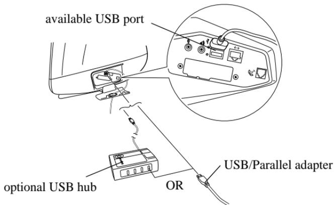
If you're using a USB hub, plug it into the USB port on your iMac, then connect the adapter to an available USB port on the hub.
