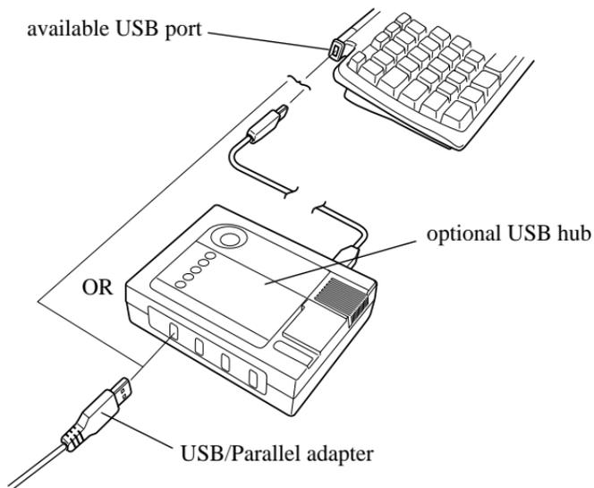
If you're using a USB hub, plug it into the USB port on the iMac keyboard, then connect the adapter to an available USB port on the hub.
