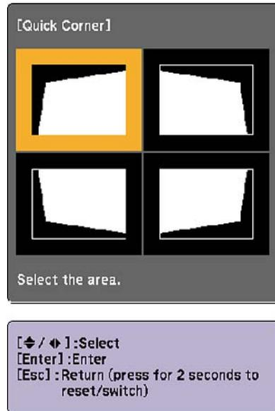
6. Use the arrow buttons on the projector or the remote control to select the corner of the image you want to adjust. Then press **Enter**.
