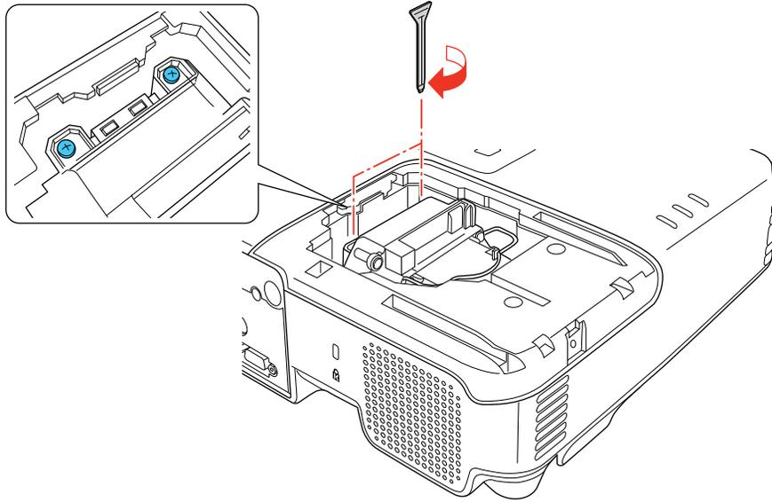
9. Replace the lamp cover and tighten the screw to secure it.
