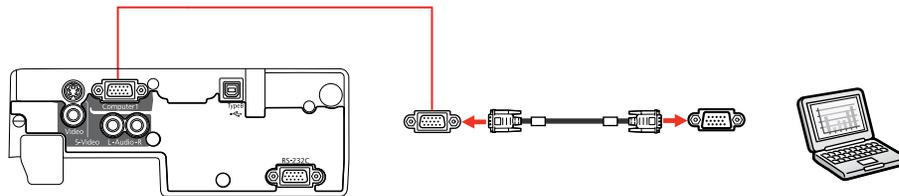
4. Tighten the screws on the VGA connectors.
