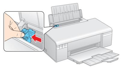
4 Load paper against the right edge guide and behind the tab, with the printable side face up.
