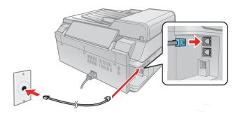
**Note:** If you're connecting to a DSL phone line, you must use a DSL filter or you won't be able to fax. Contact your DSL provider for the necessary filter.
