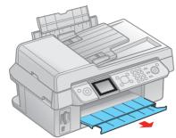
3 Squeeze the edge guide and slide it to the left. Then flip the feeder guard forward.
