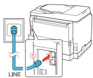
Note: If you're connecting to a DSL phone line, you must use a DSL filter or you won't be able to fax. Contact your DSL provider for the necessary filter.
