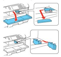
**2** Remove tape and protective materials from the second paper cassette, and install as shown.
