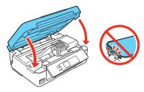
6 Press OK to prime the ink delivery system. Priming takes about 4 minutes.
