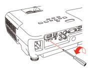
2 Connect the wireless LAN module to the projector's **USB-A** (flat) port.
