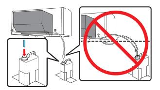
Make sure that the tube sits above the yellow line indicated on the outside of the bottle. If the tube is too long, cut the end to the appropriate length.
