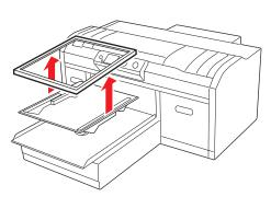
Make sure the height adjustment lever is at the "**P**" position.
