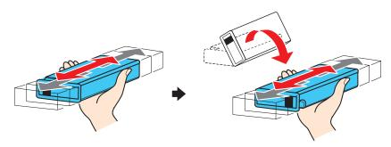
Open the ink covers and install each cartridge into the correct slot for its color.
