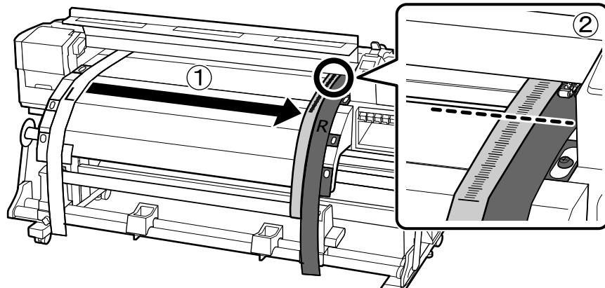
7. Make sure all four of the mounting screws are loose. To make adjustments, turn the adjustment screw counterclockwise to move the line back, and turn it clockwise to move the line forward. The line will move approximately 1 mm with each turn of the screw. Continue to turn the silver adjustment screw until the measurements are the same.
