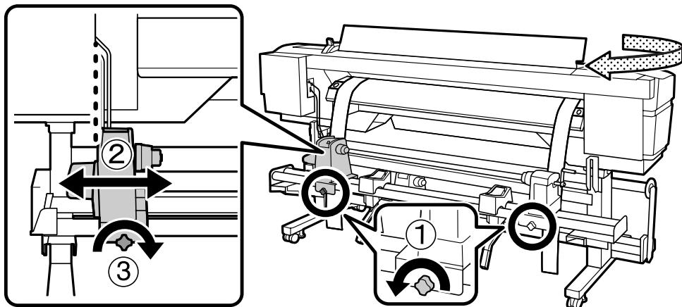
7. If the roll holder handle shaft is pushed in, rotate the handle towards you (counterclockwise) until it no longer turns.
