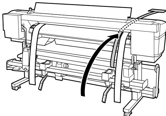
11. Place the alignment tool next to the left adjustment guide and line them up at the front and back of the printer.
