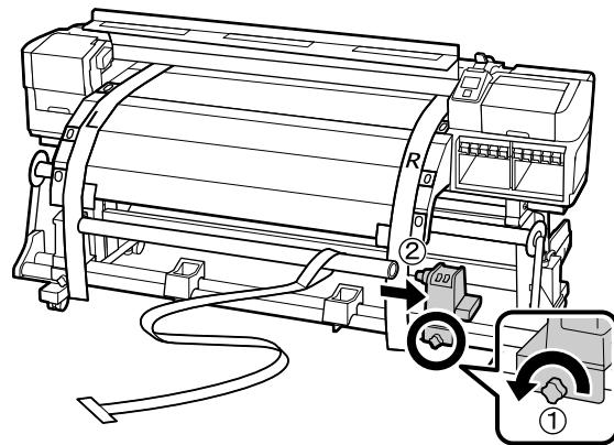
12. Remove the roll core and the alignment tool.
