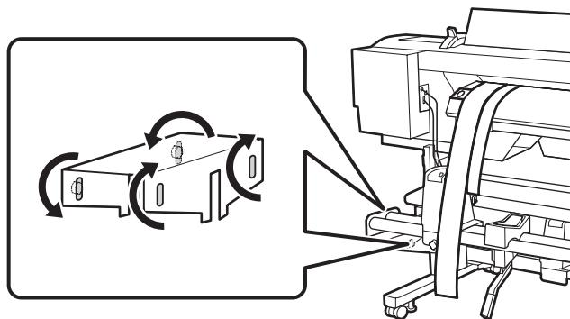
16. At the front of the printer, remove the counterweight from the alignment tool.
