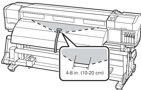
4. Feed the media by pressing the ▶ button, until the leading edge of the paper tape reaches the roll core on the auto take-up reel.
