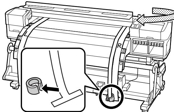
17. From the back of the printer, remove the alignment tool.
