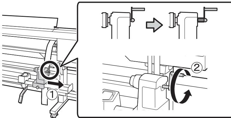
8. Slide the included 64-inch roll core into the loop at the end of the alignment tool:
