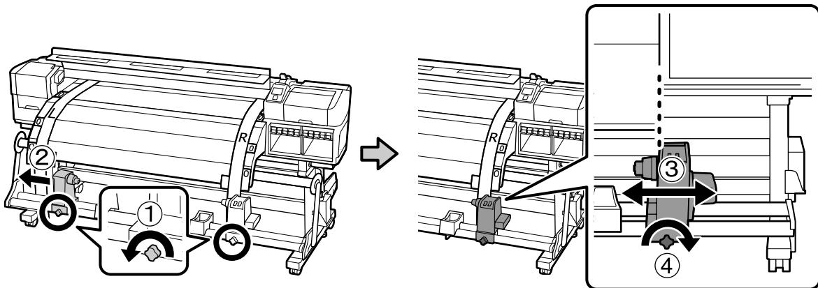
2. Load the roll core with the alignment tool onto the roll holder:
