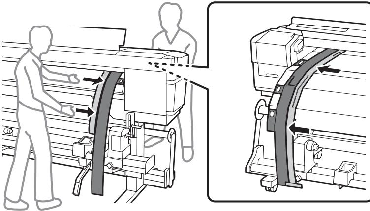
12. Attach the counterweight to the alignment tool to keep it stretched taut. Note the location where it crosses the front of the white line on the platen.
