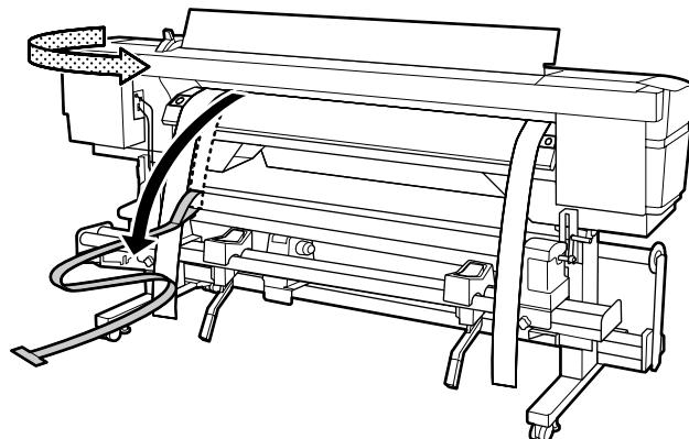
18. Loosen the roll holder fixing screw and move the right roll holder.
