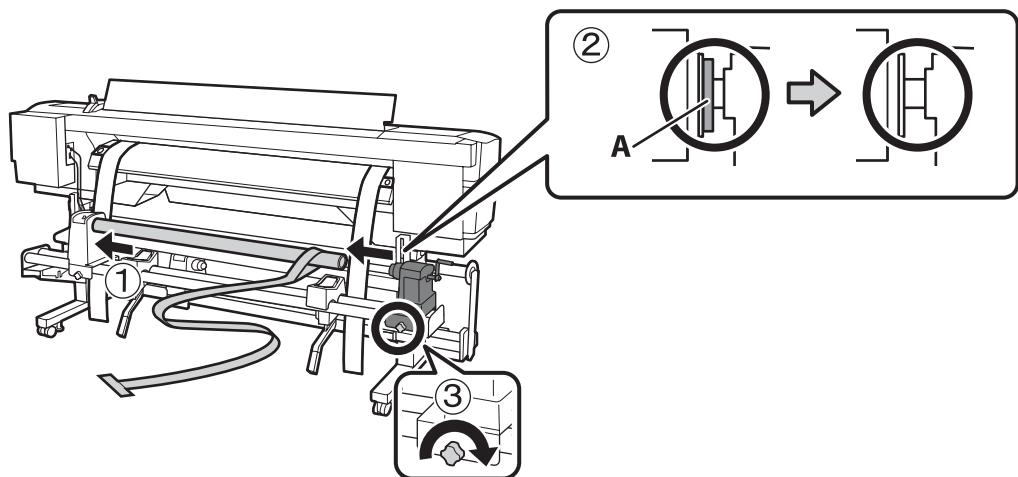
10. Slide the alignment tool to the right side of the roll core and feed it into the printer.
