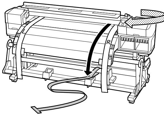
11. Loosen the roll holder fixing screw and move the right roll holder.
