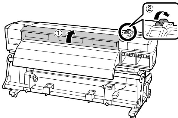
2. From the back of the printer, feed the left and right adjustment guides through the paper path as shown:
