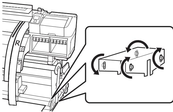
9. At the back of the printer, remove the counterweight from the alignment tool.
