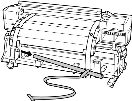
13. Remove the alignment tool from the roll core, then remove the adjustment guides from the printer.
