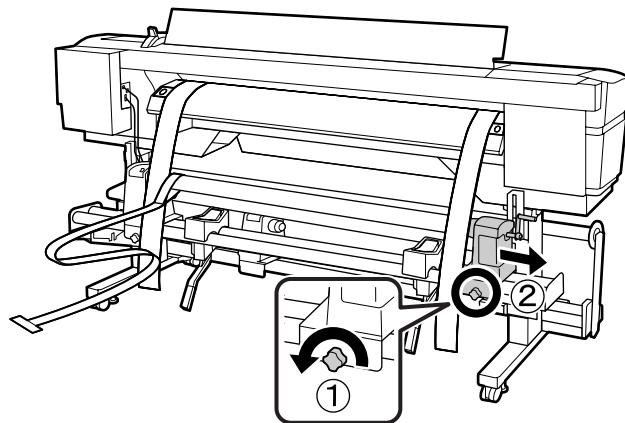
19. Remove the roll core and the alignment tool.
