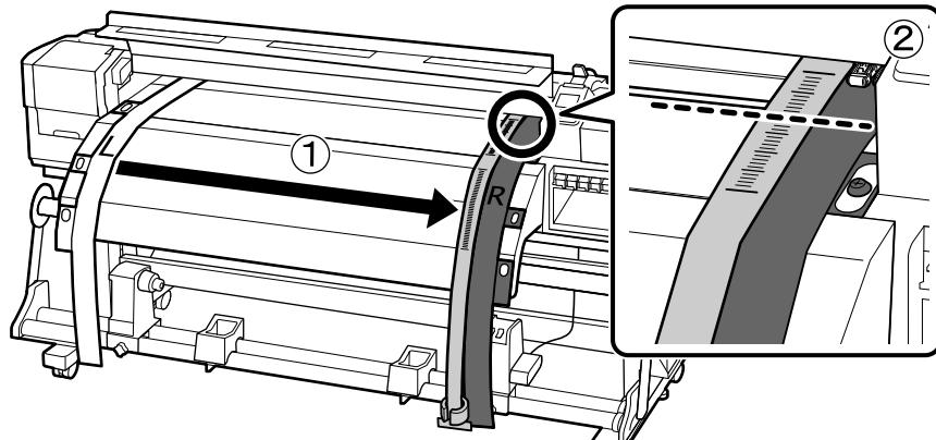
14. Make sure all four of the mounting screws are loose. To make adjustments, have a person at the back of the printer turn the silver adjustment screw. Turn the screw counterclockwise to move the line back, and turn it clockwise to move the line forward. The line will move approximately 1 mm with each turn of the screw. Continue to turn the silver adjustment screw until the measurements are the same.
