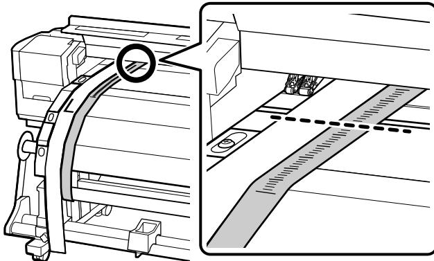
6. Lift up the alignment tool and slide it to the other side of the printer, next to the right adjustment guide. Line up the alignment tool and the adjustment guide at the front and back of the printer.
