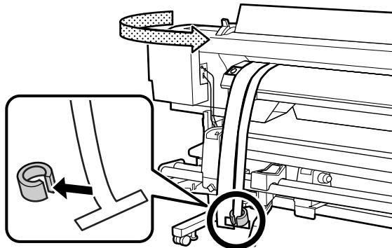
10. At the front of the printer, remove the alignment tool.
