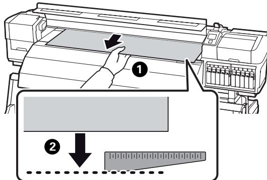
2. Cut off about 24 inches (60 cm) of paper tape and attach it to the media using adhesive tape.
