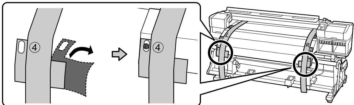
6. At the back of the printer, align the left side of the roll holder with the left side of the printer as shown. Then tighten the roll holder fixing screw to secure it in place.
