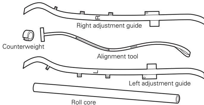
Before you begin the parallel adjustment procedure, make sure the printer is leveled and on a level surface. Carefully unroll the adjustment guides.
