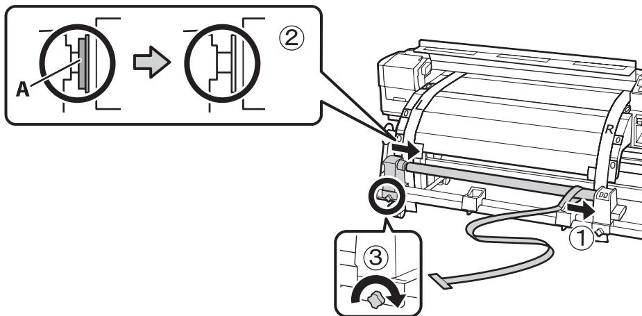
3. From the front of the printer, move the alignment tool to the left side and feed it through the paper path as shown:
