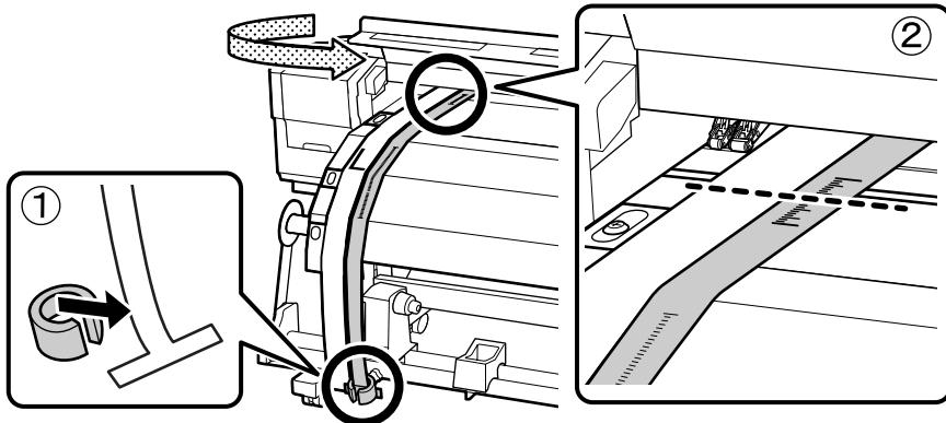
13. Lift up the alignment tool and slide it to the other side of the printer, next to the right adjustment guide. Line up the alignment tool and the adjustment guide at the front and back of the printer.
