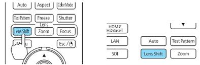
Press the arrow buttons on the remote control or projector to adjust the position.
