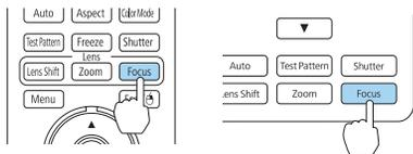
Press the left and right arrow buttons on the remote control or projector to adjust the focus.
