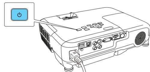
**Note:** To shut down the projector, press the power button twice, then unplug it. You don't have to wait for the projector to cool down.
