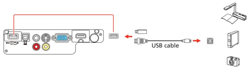
If you connect a digital camera, USB flash drive, or USB storage device, you can use the projector's **PC Free** feature. You can also connect other Epson document cameras to the projector. See the online *User's Guide* for details.
