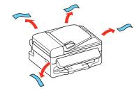
2 Lift up the scanner unit and remove all protective materials from inside the product.
