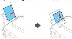
Slide the edge guide against the paper, but not too tightly, and flip the feeder guard back.
