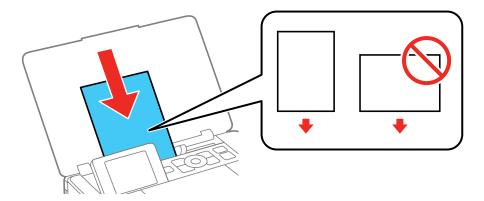
**Note:** To load envelopes, insert the envelopes printable side up and flap edge left.
