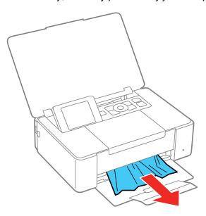
4. Open the inner cover and carefully remove any jammed paper.
