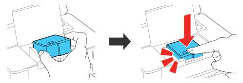
**Caution:** Make sure to insert the ink cartridge in the correct direction or you may damage the product.
