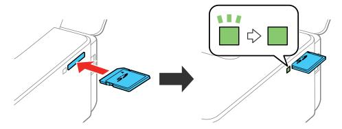
**Note:** Do not force the card all the way into the slot. Insert it only until it meets resistance.
