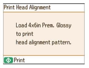
6. Press the ♦ start button to print an alignment sheet.
