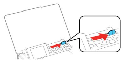
2. Load paper, glossy or printable side up and short edge first, against the left side of the paper feed slot.
