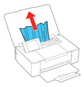
3. If necessary, carefully pull out any jammed paper from the front.
