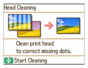
6. Press the ♦ start button to clean the print head. You see a print head cleaning message on the LCD screen during the cleaning cycle.
