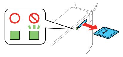
2. Pull the memory card straight out of its slot.
