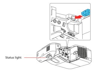
Press the power button on the projector or remote control. The projector beeps, and the Status light flashes blue and then stays on.
