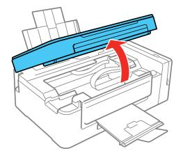
**Caution:** Do not touch the flat white cable inside the printer. Do not lift the scanner unit while the document cover is open.
