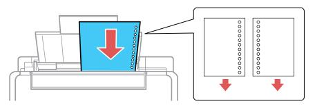
6. Slide the edge guide against the paper, but not too tightly. Then flip the feeder guard back.
