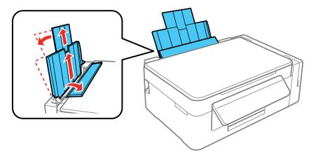
2. Pull out the output tray and open the paper stopper on the end.
