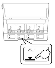
**Caution:** If the ink level is below the lower line on the ink tank, fill it to the upper line on the ink tank. Continued use of the product when the ink level is below the lower line on the tank could damage the product.
