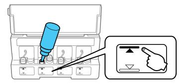
5. If any ink remains in the ink bottle after filling the ink tank, replace the bottle cap and tighten it securely. Store the ink bottle upright for later use.
