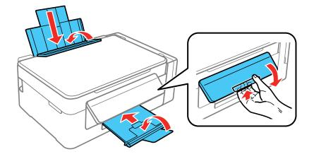
**Caution:** Do not lower the control panel without first squeezing the release bar or you may damage your product.
