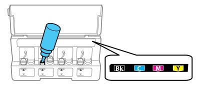
3. Unscrew the cap on the bottle and remove it. Do not dispose of the cap so you can use it to close the bottle later, if necessary. Then remove the bottle cap and carefully remove the protective seal (avoid touching the ink underneath the seal). Close the bottle cap tightly.
