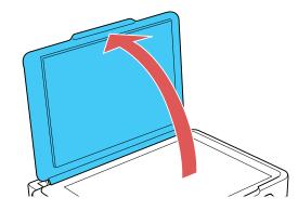
2. Place your original facedown on the scanner glass with the top facing into the corner. Slide the original to the edges of the indicated corner.
