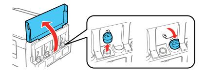
**Note:** Make sure the color of the ink tank label matches the ink color you want to refill, and only remove the cap from that ink tank. Be careful not to spill any ink.
