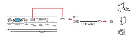
If you connect a digital camera, USB flash drive, or USB storage device, you can use the projector's PC Free feature. You can also connect Epson document cameras to the projector. See the online User's Guide for details.
