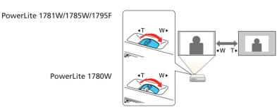
4 PowerLite 1781W/1785W/1795F: To sharpen the image, press the Focus buttons on the projector or remote control.
