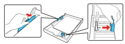
Insert the paper cassette. Push it firmly into the printer.
