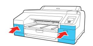
2 Remove the packing materials inside the ink compartments.
