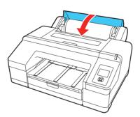
**Note:** Always keep the roll paper cover closed to prevent dust from entering the printer.
