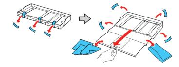
Pull out the paper cassette and open the top cover. Remove all packing materials and tape from inside the product, then close the top cover.
