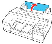
6 Place the roll paper in the printer as shown (the black end of the spindle goes on the left).
