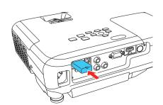
Attach the included wireless LAN module cover and secure it using the screw you removed.
