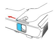
4 Press the (b) power button on the projector or remote control. The projector beeps, the Status light flashes blue, and then stays on.
