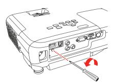
Insert the included wireless LAN module into the **USB-A** port.
