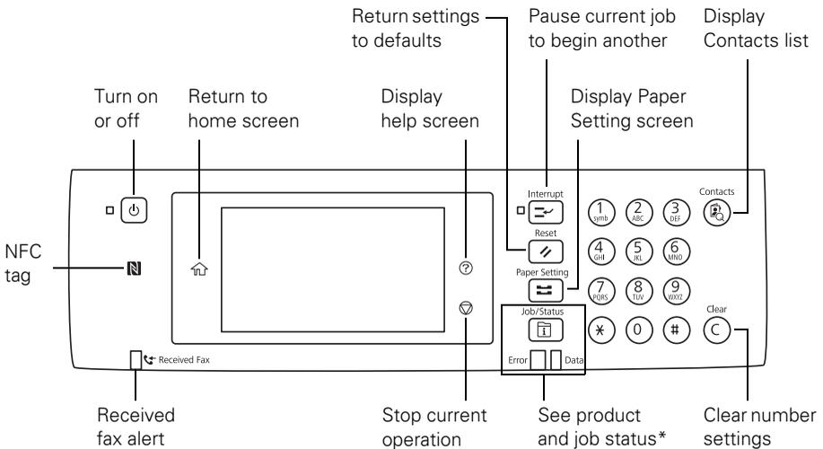
\* The Error light flashes or turns on when an error occurs. The Data light flashes when the product is processing data and turns on when there are print jobs waiting.
