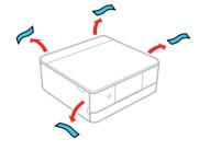
2 Lift up the scanner unit. Remove all protective materials from inside the product.
