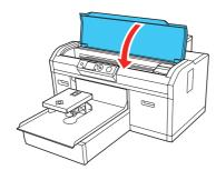
The printer starts a cleaning cycle. This takes about 10 minutes. The LCD displays a message when cleaning is complete.
