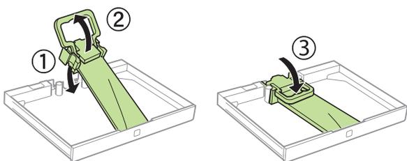
**Note:** Make sure the ink pack is fully inserted and level with the top of the ink pack tray.
