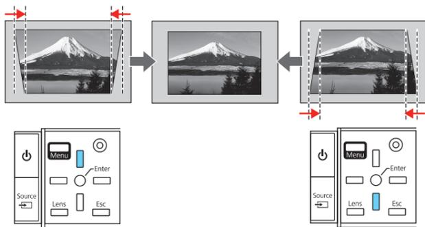
**Note:** Using the keystone adjustment can affect the size and effective resolution of your image. If possible, change the position of your projector to eliminate the keystone effect and use the lens shift option to position the image as necessary.
