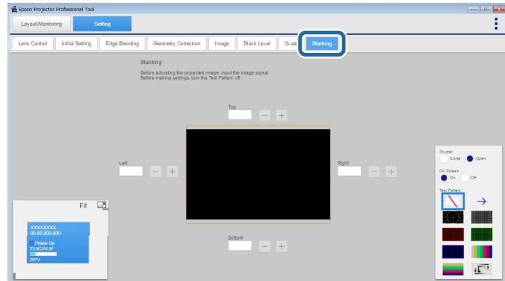
**Note:** When no input signal is received, you cannot adjust the **Blanking** settings.
