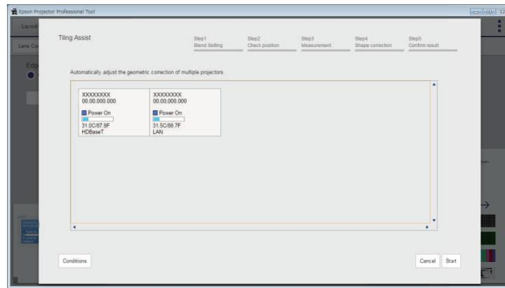
5. If a specified **Edge Blending** value is incorrect, the **Blend Setting** screen appears. Adjust the **Edge Blending** values as necessary.
