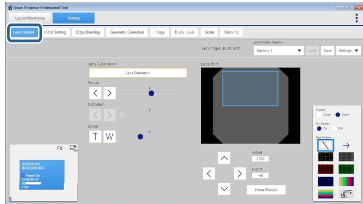
Depending on the type of lens you installed, the available features or adjustment ranges may vary. And depending on the firmware version, the image may appear longer horizontally in the preview image than in the actual image.
