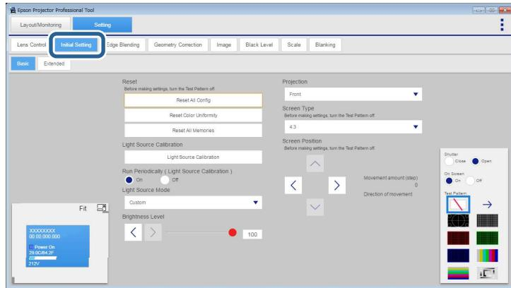
You can adjust the settings for multiple projectors or groups on the **Initial Setting** tab. If you select different projector models, you can adjust only settings that are available on all selected projectors.
