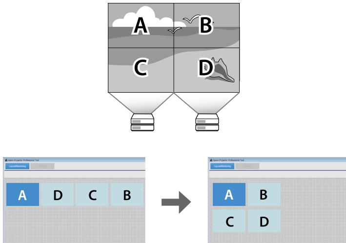
When you have finished making adjustments of the layout, select the **Save** button to save the project.
