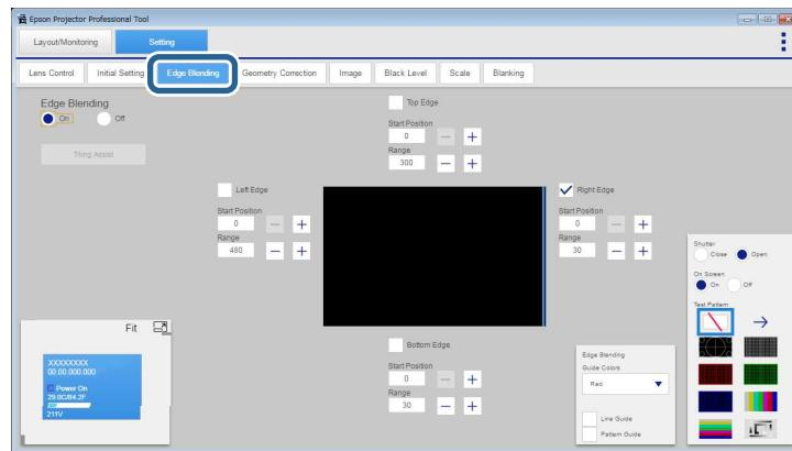
Before using the **Edge Blending** settings, select the **Image** tab and select **Multi-Projection** as the **Color Mode** setting.
