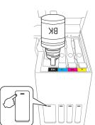
**5** When the ink tank is full, remove the ink bottle and replace the bottle cap. Place the remaining ink aside; you will need it later.
