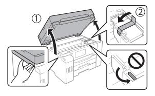
**Caution:** The printer ships with the transportation lock in the printing position. Do not move the transportation lock from the printing position.
