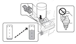
**Note:** If ink does not flow from the bottle, lift and reinsert the bottle.
