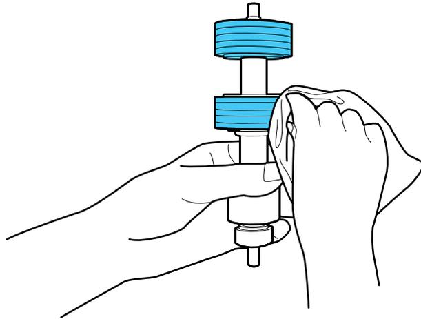
**Caution:** Use only a genuine Epson cleaning kit or soft, moist cloth to clean the roller; using a dry cloth may damage the surface of the roller. Do not spray cleaners directly inside the product; always spray cleaners on a cleaning cloth to slightly dampen the cloth. Wipe off any excess cleaner with a dry, lint-free cloth.
