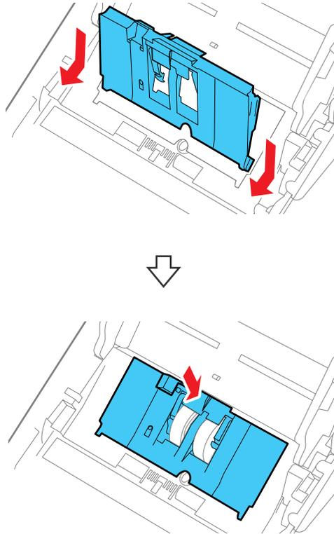
**Note:** If you are not able to close the cover, the roller is not installed correctly. Remove the roller unit and reinstall it, then try to close the cover again.
