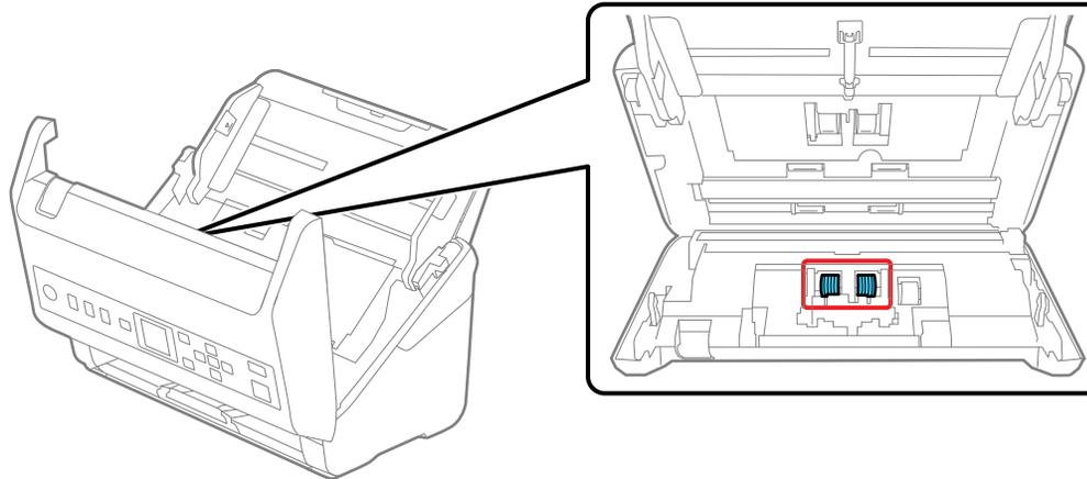
7. Squeeze the tabs on the sides of the separation roller cover and open the cover.
