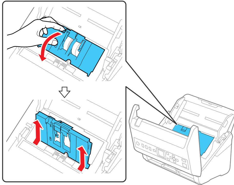
14. Pull down the tab on the pickup roller and slide the roller to the right to remove it.
