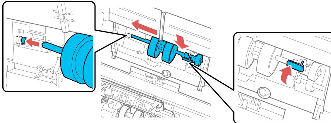
8. Align the bottom edge of the pickup roller cover into the notches as shown and press it down until it clicks into place.
