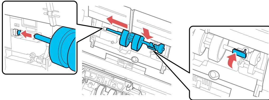
17. Align the bottom edge of the pickup roller cover into the notches as shown and press it down until it clicks into place.
