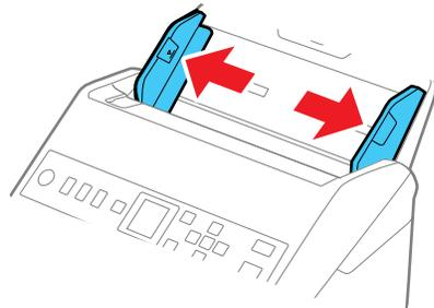
4. Load envelopes vertically in the input tray with the printed side down and the flap facing as shown. Slide in the envelopes until they meet resistance. Skip to step 7.
