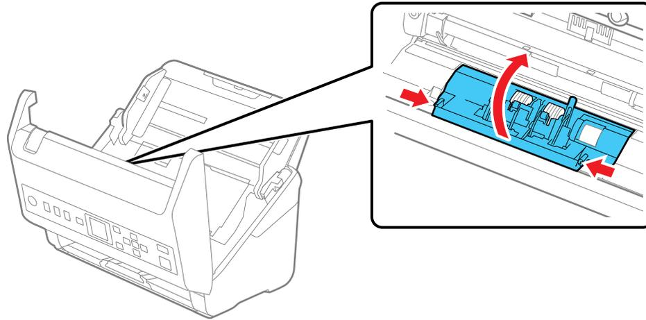
8. Slide the separation roller to the left and remove it.
