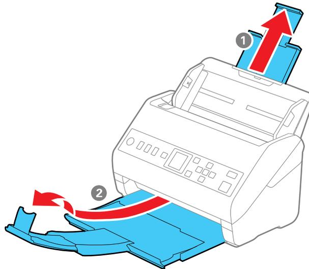
**Note:** If you are loading originals that are 15.5 inches (393.8 mm) or longer, do not pull out the input or output tray extensions and do not open the stopper.
