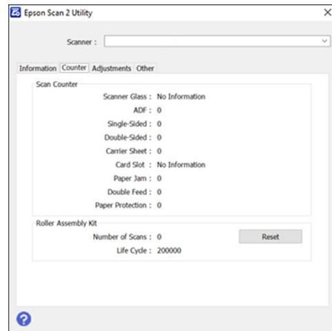
4. If the number in the **Number of Scans** field exceeds the number displayed as the **Life Cycle** of the rollers, it is time to replace the rollers.
