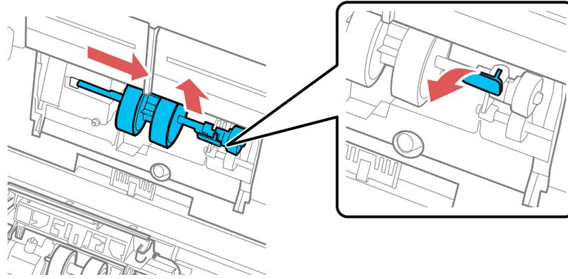
7. To install the new pickup roller, align the notches on the roller unit and slide it to the left. Press up on the tab to secure the roller.
