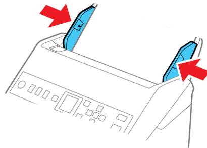
**Note:** If you are scanning originals that are 15.5 inches (393.8 mm) or longer, support the original as it enters into and ejects from the scanner as shown and use the following resolutions:
