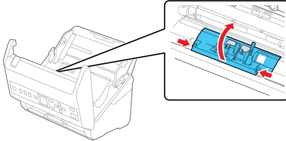
10. Slide the separation roller to the left and remove it.
