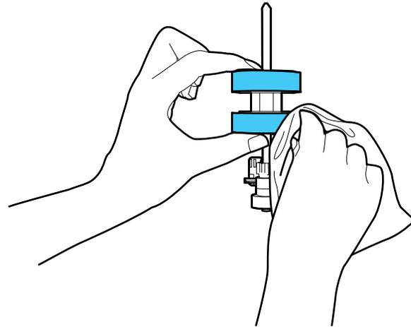
**Caution:** Use only a genuine Epson cleaning kit or soft, moist cloth to clean the roller; using a dry cloth may damage the surface of the roller.
