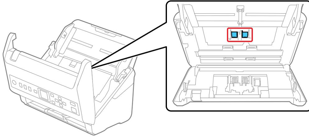
13. Press down on the pickup roller cover latch and pull up the cover to remove it.
