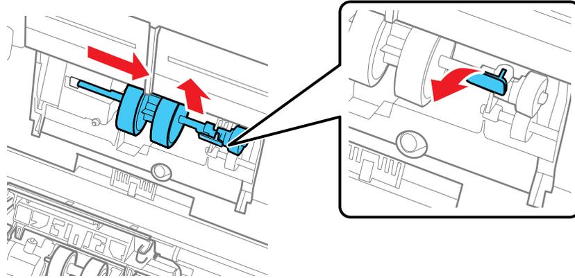
15. Wipe off any dust or dirt on the pickup roller using a genuine Epson cleaning kit or a soft, moist cloth.
