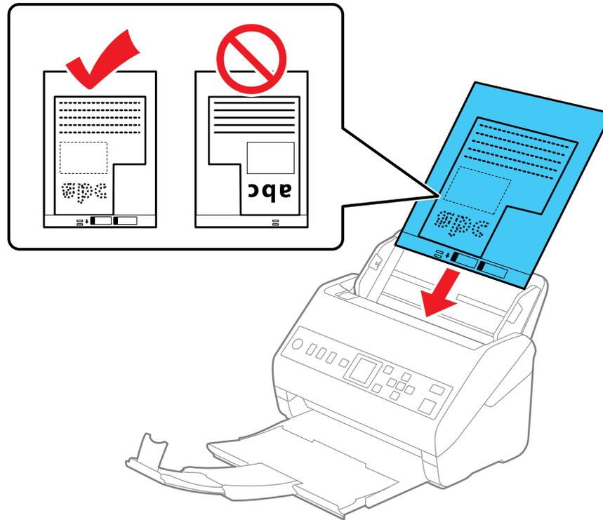
7. Slide the edge guides against the edges of the envelope or carrier sheet.
