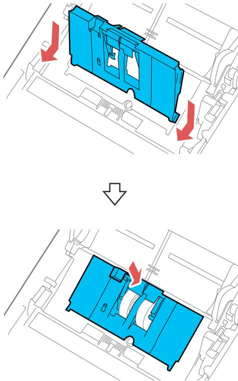
**Note:** If you are not able to close the cover, the pickup roller is not installed correctly. Remove the roller unit and reinstall it, then try to close the cover again.
