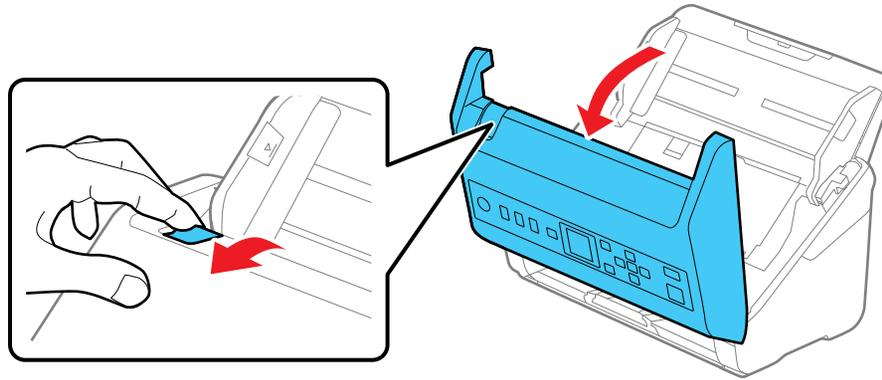
4. Gently pull out any jammed originals from inside the scanner.
