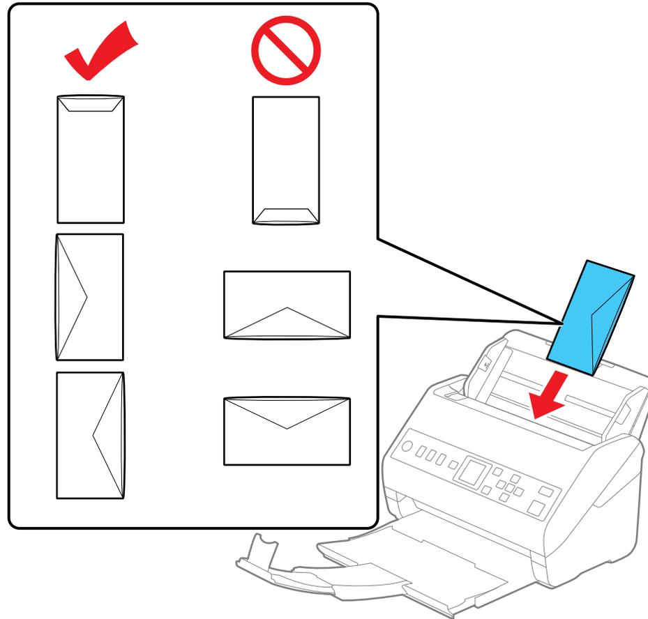
5. Do one of the following to load photos, or folded or irregularly shaped originals using a carrier sheet:
