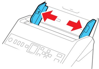
4. Load the originals in the center of the input tray in descending order of paper size with the widest at the back and the narrowest at the front. Slide them in until they meet resistance. Make sure the printed sides are facedown and the top edges are slightly angled in the input tray.
