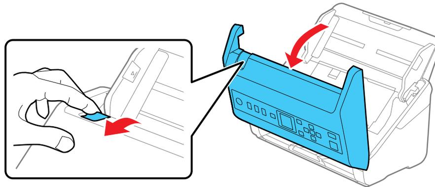
5. Press down on the pickup roller cover latch and pull up the cover to remove it.
