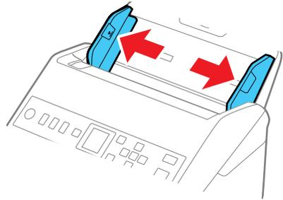
3. Load plastic or laminated cards (printed side down and long edge first) into the input tray horizontally, and slide them in until they meet resistance.
