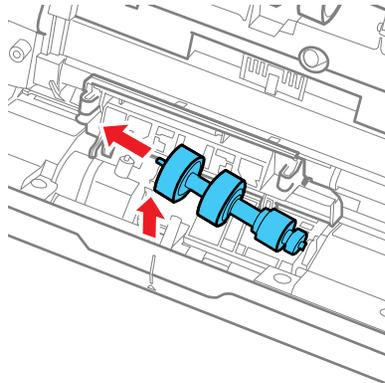
9. Wipe off any dust or dirt on the separation roller using a genuine Epson cleaning kit or a soft, moist cloth.
