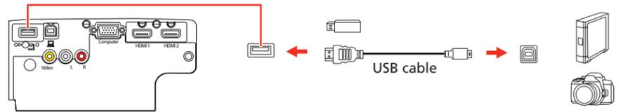
If you connect a digital camera, USB flash drive, or USB storage device, you can use the projector's PC Free feature. See the online *User's Guide* for details.
