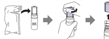
**Caution:** Do not shake or squeeze the ink bottle. Do not touch the top of the ink bottle after its cap is removed.
