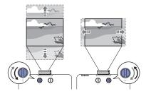
2. If the projector is on a table, you can level the image by turning any of the projector's adjustable feet.
