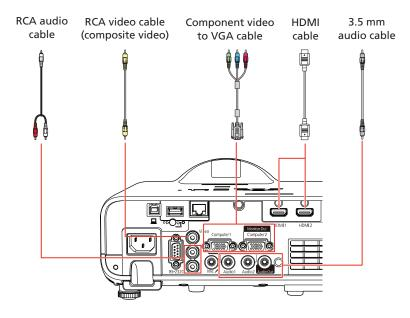
**Note:** If you connected a streaming device to an HDMI port, you can also connect it to the projector's **USB-A** (flat) port for power.
