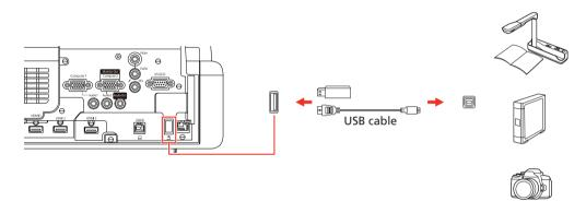
If you connect a digital camera, USB flash drive, or USB storage device, you can use the projector's PC Free feature. You can also connect other Epson document cameras to the projector. See the online *User's Guide* for details.
