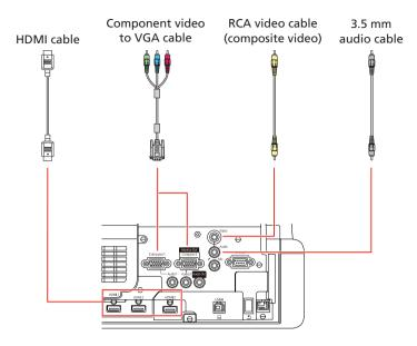
**Note:** If you connected a streaming device to an HDMI port, you can also connect it to the projector's **USB-A** (flat) port for power.
