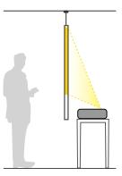
Wherever you set up the projector, make sure to position it squarely in front of the screen, not at an angle.
