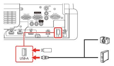
**Note:** Use the USB cable supplied with or specified for use with your device. Do not connect a USB hub or a USB cable longer than 10 feet (3 m), or the device may not operate correctly.
