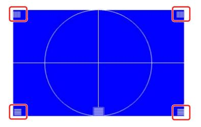
**Note:** If any areas are out of focus, use the focus lever to adjust the focus until the corners appear the same.
