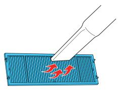
**Caution:** Do not rinse the air filter in water, or use any detergent or solvent to clean it. Do not use canned air; the gases may leave a flammable residue, or push dust and debris into the projector's optics or other sensitive areas.
