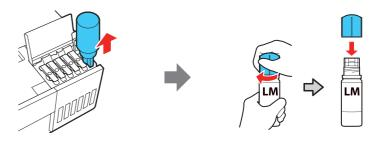
**Note:** Do not leave the ink bottle inserted; otherwise the bottle may be damaged or ink may leak. Once the ink tank is full, do not remove and reinsert the ink bottle or ink may spill.
